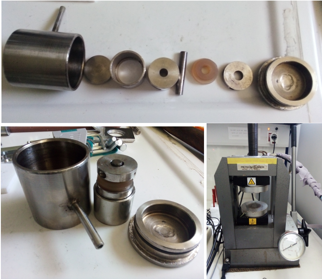
Figure 1: Top: Pieces used for the press: bottom part of the outer chamber, bottom part of the inner chamber, inner chamber, cylinder with the hole of diameter 8mm, stick with the diameter 8 mm, rubber bands, upper load, upper lid of the outer chamber. Bottom Left: Assembled parts. Bottom Right: Hot press. The lever on the right is used to apply pressure.
